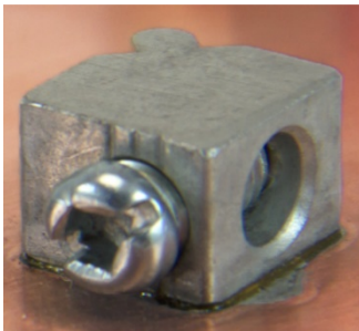
B6A-PCB-45(-RS) SMT mode horizontal screw axis AWG 6-14 65A 75C (0.50" X 0.53" contact surface)
