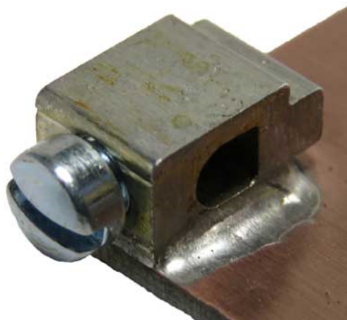
Figure 12. Shows a strong fillet on the counterclockwise torque lateral edge line.
